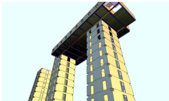
Figure 2 - Half a floor lifted into place
